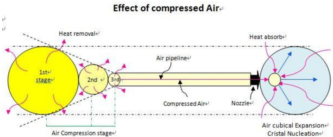
Most conventional air/water snowmaking systems create pressures of roughly 80 to 100 psi. The smaller the volume to which the air is compressed, however, the greater amount of mechanical energy is released when it returns to normal atmospheric pressure -and the more heat is absorbed upon release of pressure.
